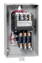
Non-reversing motor starter, Size 1 3/4, Three phase full voltage, Amb. compensate bimetal OLR, Contactor amp rating 40A, Non-combination type, Enclosure type 1, Indoor general purpose use
