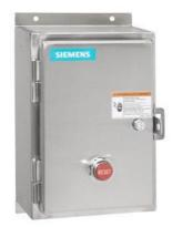
Non-reversing motor starter, Size 1 3/4, Three phase full voltage, Amb. compensate bimetal OLR, Contactor amp rating 40A, Non-combination type, Encl. type 4X 304 S. Steel, Water/dust tight noncorrosive
