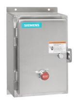
Non-reversing motor starter, Size 1 3/4, Three phase full voltage, Amb compensate bimetal OLrelay Contactor amp rating 40Amp 550/575 600 50/60HZ coil, Non-combination type, Enclosure type 4X 304 S-steel, Water/dust tight noncorrosive
