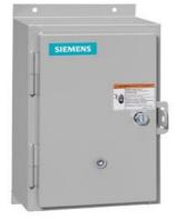
Non-reversing motor starter, Size 2, Single Phase, 2-Pole, Amb. compensate bimetal OLR, Contactor amp rating 45A, 110V 50Hz / 120V 60Hz coil, Noncombination type, Enclosure type 12, Dust/drip proof for indoors
