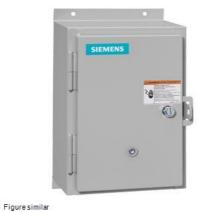
Non-reversing motor starter, Size 2, Single Phase, 2-Pole, Amb. compensate bimetal OLR, Contactor amp rating 45A, Non-combination type, Enclosure type 12, Dust/drip proof for indoors
