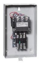
Non-reversing motor starter, Size 2, Single Phase, 2-Pole, Amb. compensate bimetal OLR, Contactor amp rating 45A, 24VAC 50-60Hz coil, Non-combination type, Enclosure type 1, Indoor general purpose use
