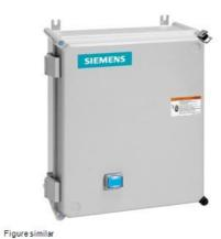
Non-reversing motor starter, Size 2, Single Phase, 2-Pole, Amb. compensate bimetal OLR, Contactor amp rating 45A, Non-combination type, Enclosure type 4X fiberglass, Water/dust tight noncorrosive
