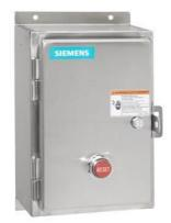
Non-reversing motor starter, Size 2, Single Phase, 2-Pole, Amb. compensate bimetal OLR, Contactor amp rating 45A, 110V 50Hz / 120V 60Hz coil, Non-combination type, Encl. type 4X 304 S. Steel, Water/dust tight noncorrosive
