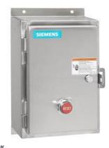
Non-reversing motor starter, Size 2, Single Phase, 2-Pole, Amb. compensate bimetal OLR, Contactor amp rating 45A, Non-combination type, Encl. type 4X 304 S. Steel, Water/dust tight noncorrosive
