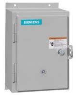
Non-reversing motor starter, Size 2, Three phase full voltage, Amb. compensate bimetal OLR, Contactor amp rating 45A, Non-combination type, Enclosure type 12, Dust/drip proof for indoors
