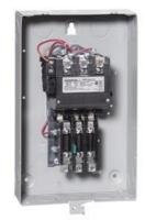
Non-reversing motor starter, Size 2, Three phase full voltage, Amb. compensate bimetal OLR, Contactor amp rating 45A, 208VAC 60Hz coil, Non-combination type, Enclosure type 1, Indoor general purpose use
