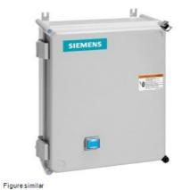
Non-reversing motor starter, Size 2, Three phase full voltage, Amb. compensate bimetal OLR, Contactor amp rating 45A, 110V 50Hz / 120V 60Hz coil, Non-combination type, Enclosure type 4X fiberglass, Water/dust tight noncorrosive
