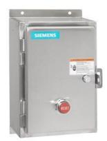
Non-reversing motor starter, Size 2, Three phase full voltage, Amb. compensate bimetal OLR, Contactor amp rating 45A, 240V 50Hz / 277V 60Hz coil, Noncombination type, Encl. type 4X 304 S. Steel, Water/dust tight noncorrosive
