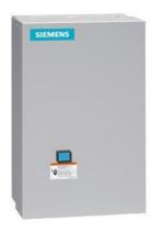
Non-reversing motor starter, Size 2, Three phase full voltage, Amb. compensate bimetal OLR, Contactor amp rating 45A, 110V 50Hz / 120V 60Hz coil, Non-combination type, Enclosure type 1, Indoor general purpose use
