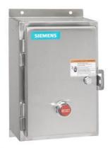
Non-reversing motor starter, Size 2, Three phase full voltage, Amb. compensate bimetal OLR, Contactor amp rating 45A, 110V 50Hz / 120V 60Hz coil, Non-combination type, Encl. type 4X 304 S. Steel, Water/dust tight noncorrosive
