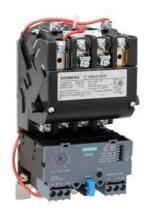
Non-reversing motor starter Size 2 Three phase full voltage Solid-state overload relay OLRelay amp range 13-52a 110-120/220-240VAC 60HZ coil Combination type No enclosure
