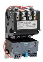
Non-reversing motor starter Size 2 Three phase full voltage Solid-state overload relay OLRelay amp range 13-52a 110VAC 50HZ / 120VAC 60HZ coil Combination type No enclosure
