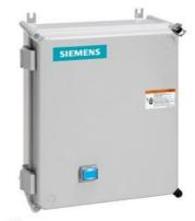
Non-reversing motor starter, Size 2, Three phase full voltage, Solid-state overload relay, OLR amp range 13-52A, 110V 50Hz / 120V 60Hz coil, Non-combination type, Enclosure type 4X fiberglass, Water/dust tight noncorrosive, Standard width enclosure
