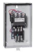
Non-reversing motor starter, Size 2 1/2, Single Phase, 2-Pole, Amb. compensate bimetal OLR, Contactor amp rating 60A, Non-combination type, Enclosure type 1, Indoor general purpose use
