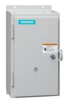
Non-reversing motor starter, Size 2 1/2, Three phase full voltage, Amb compensate bimetal OLrelay Contactor amp rating 60Amp 110V 50HZ / 120V 60HZ coil, Noncombination type, Enclosure type 12, Dust/drip proof for indoors
