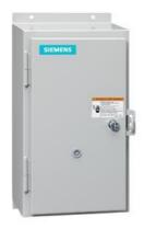
Non-reversing motor starter, Size 2 1/2, Three phase full voltage, Amb. compensate bimetal OLR, Contactor amp rating 60A, 110V 50Hz / 120V 60Hz coil, Non-combination type, Enclosure type 12, Dust/drip proof for indoors
