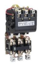
Non-reversing motor starter, Size 2 1/2, Three phase full voltage, Amb. compensate bimetal OLR, Contactor amp rating 60A, 110 120/220 240VAC 60Hz coil, Non-combination type, Enclosure type (open), No enclosure
