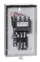
Non-reversing motor starter, Size 2 1/2, Three phase full voltage, Amb. compensate bimetal OLR, Contactor amp rating 60A, Non-combination type, Enclosure type 1, Indoor general purpose use
