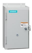
Non-reversing motor starter, Size 2 1/2, Three phase full voltage, Solid-state overload relay, OLRelay amp range 25-100A, 550/575 600 50/60HZ coil, Non-combination type, Enclosure type 12, Dust/drip proof for indoors, Standard width enclosure
