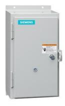
Non-reversing motor starter, Size 2 1/2, Three phase full voltage, Solid-state overload relay, OLR amp range 25-100A, Non-combination type, Enclosure type 12, Dust/drip proof for indoors, Standard width enclosure
