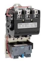
Non-reversing motor starter Size 2 1/2 Three phase full voltage Solid-state overload relay OLRelay amp range 25-100A 550/575-600 50/60HZ coil Combination type No enclosure
