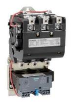
Non-reversing motor starter Size 2 1/2 Three phase full voltage Solid-state overload relay OLRelay amp range 25-100A 240VAC 50HZ / 277VAC 60HZ coil Combination type No enclosure
