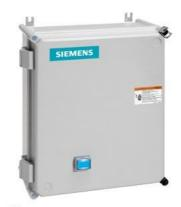
Non-reversing motor starter, Size 2 1/2, Three phase full voltage, Solid-state overload relay, OLR amp range 25-100A, Non-combination type, Enclosure type 4X fiberglass, Water/dust tight noncorrosive, Standard width enclosure
