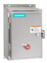
Non-reversing motor starter, Size 2 1/2, Three phase full voltage, Solid-state overload relay, OLR amp range 25-100A, 208VAC 60Hz coil, Non-combination type, Encl. type 4X 304 S. Steel, Water/dust tight noncorrosive, Standard width enclosure
