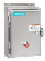
Non-reversing motor starter, Size 2 1/2, Three phase full voltage, Solid-state overload relay, OLR amp range 25-100A, Non-combination type, Encl. type 4X 304 S. Steel, Water/dust tight noncorrosive, Standard width enclosure
