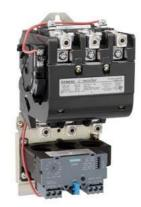
Non-reversing motor starter Size 3 Three phase full voltage Solid-state overload relay OLRelay amp range 25-100A 220-240/440-480VAC 60HZ coil Combination type No enclosure
