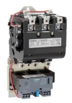
Non-reversing motor starter Size 3 Three phase full voltage Solid-state overload relay OLRelay amp range 25-100A 24Vdc coil Combination type No enclosure
