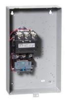
Non-reversing motor starter, Size 3, Three phase full voltage, Solid-state overload relay, OLR amp range 25-100A, 24VDC coil, Non-combination type, Enclosure type 1, Indoor general purpose use, Standard width enclosure
