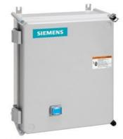
Non-reversing motor starter, Size 3, Three phase full voltage, Solid-state overload relay, OLR amp range 25-100A, 110V 50Hz / 120V 60Hz coil, Non-combination type, Enclosure type 4X fiberglass, Water/dust tight noncorrosive, Standard width enclosure
