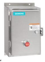
Non-reversing motor starter, Size 3, Three phase full voltage, Solid-state overload relay, OLR amp range 25-100A, 110V 50Hz / 120V 60Hz coil, Non-combination type, Encl. type 4X 304 S. Steel, Water/dust tight noncorrosive, Standard width enclosure
