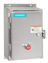
Non-reversing motor starter Size 3 Three phase full voltage Solid-state overload relay OLRelay amp range 25-100A 240VAC 50HZ / 277VAC 60HZ coil Combination type Water/dust tight non-corrosive
