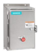
Non-reversing motor starter Size 3 Three phase full voltage Solid-state overload relay OLRelay amp range 25-100A 24Vdc coil Combination type Water/dust tight non-corrosive
