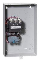
Non-reversing motor starter Size 3 Three phase full voltage Solid-state overload relay OLRelay amp range 25-100A 220-240/440-480VAC 60HZ coil Combination type Indoor general purpose use
