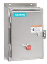
Non-reversing motor starter Size 3 Three phase full voltage Solid-state overload relay OLRelay amp range 25-100A 110-120/220-240VAC 60HZ coil Combination type Water/dust tight non-corrosive
