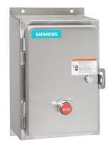
Non-reversing motor starter Size 3 Three phase full voltage Solid-state overload relay OLRelay amp range 25-100A 380-440/440-480V 50/60HZ coil Combination type Water/dust tight non-corrosive
