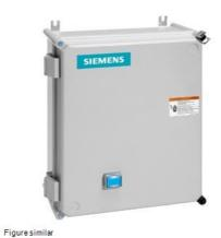
Non-reversing motor starter, Size 3 1/2, Three phase full voltage, Amb. compensate bimetal OLR, Contactor amp rating 115A, 110V 50Hz / 120V 60Hz coil, Non-combination type, Enclosure type 4X fiberglass, Water/dust tight noncorrosive
