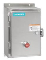
Non-reversing motor starter, Size 3 1/2, Three phase full voltage, Amb. compensate bimetal OLR, Contactor amp rating 115A, 208VAC 60Hz coil, Noncombination type, Encl. type 4X 304 S. Steel, Water/dust tight noncorrosive
