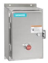
Non-reversing motor starter, Size 3 1/2, Three phase full voltage, Amb. compensate bimetal OLR, Contactor amp rating 115A, Non-combination type, Encl. type 4X 304 S. Steel, Water/dust tight noncorrosive
