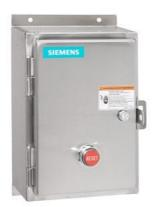
Non-reversing motor starter, Size 3 1/2, Three phase full voltage, Solid-state overload relay, OLR amp range 50-200A, 110V 50Hz / 120V 60Hz coil, Noncombination type, Encl. type 4X 304 S. Steel, Water/dust tight noncorrosive, Standard width enclosure
