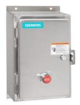
Non-reversing motor starter Size 3 1/2 Three phase full voltage Solid-state overload relay OLRelay amp range 50-200A 190-220/220-240V 50/60HZ coil Combination type Water/dust tight non-corrosive
