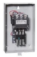
Non-reversing motor starter, Size 4, Three phase full voltage, Amb. compensate bimetal OLR, Contactor amp rating 135A, Non-combination type, Enclosure type 1, Indoor general purpose use
