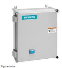
Non-reversing motor starter, Size 4, Three phase full voltage, Amb. compensate bimetal OLR, Contactor amp rating 135A, 110V 50Hz / 120V 60Hz coil, Non-combination type, Enclosure type 4X fiberglass, Water/dust tight noncorrosive
