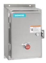
Non-reversing motor starter, Size 4, Three phase full voltage, Amb. compensate bimetal OLR, Contactor amp rating 135A, 208VAC 60Hz coil, Non-combination type, Encl. type 4X 304 S. Steel, Water/dust tight noncorrosive
