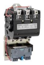
Non-reversing motor starter Size 4 Three phase full voltage Solid-state overload relay OLRelay amp range 50-200A 220-240/440-480VAC 60HZ coil Combination type No enclosure
