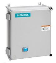
Non-reversing motor starter, Size 4, Three phase full voltage, Solid-state overload relay, OLR amp range 50-200A, Non-combination type, Enclosure type 4X fiberglass, Water/dust tight noncorrosive, Standard width enclosure
